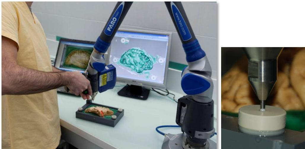
Setup overview while anatomist is scanning a specimen being dissected
